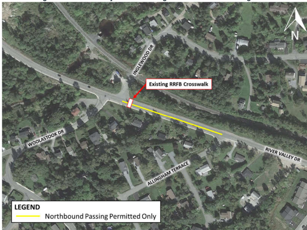
Figure 4: River Valley Drive Passing Permitted Zone Configuration
