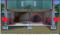
UNEQUAL PRESSURE = FOUNDATION DAMAGE PRESSION INÉGALE = FONDATION ENDOMMAGÉE
