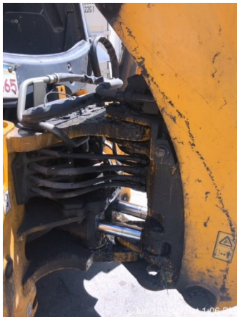
A closer look at where the excavating arm and machine are connected and pivot.
