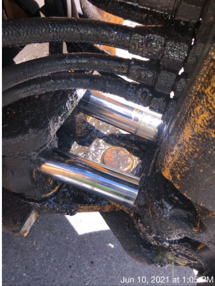
The lower king pin in between the two chrome swing pistons.
